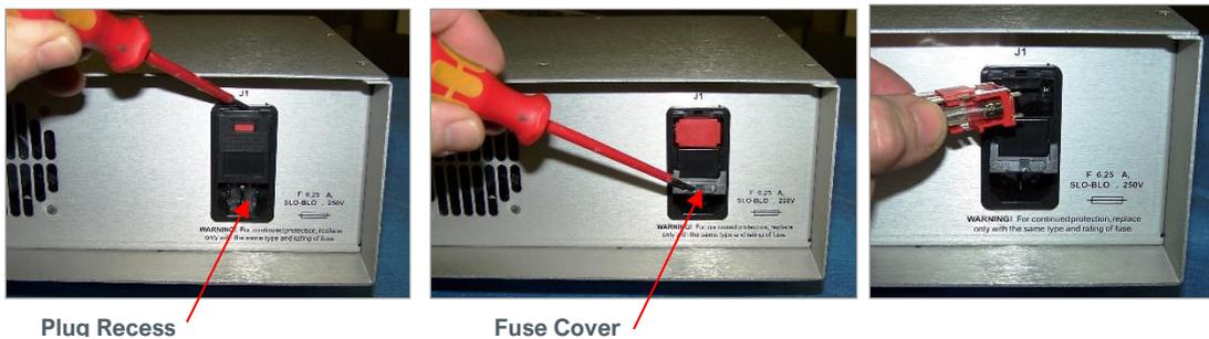
5. Slide out the blown Fuses and replace with new 6.25 Amp, slow-blow Fuses.
