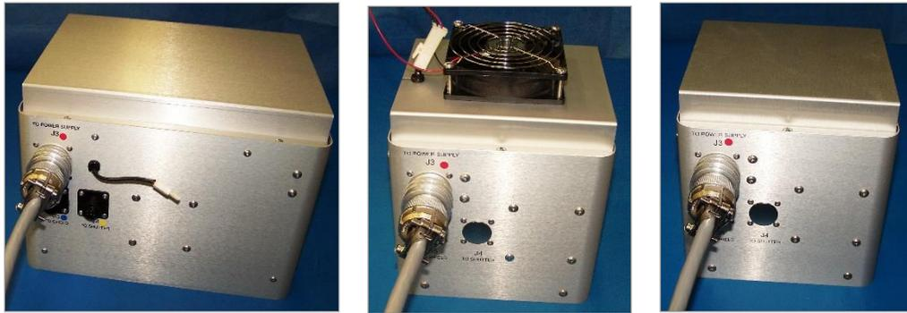
4. Connect the opposite end of the Interconnect Cable to the Lamp Power Receptacle (Figure 10) on rear panel of the Power Supply.
