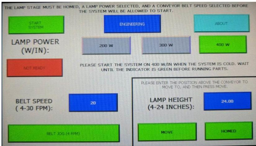
6. Press “Start System” to turn on the Conveyor, UV Lamp, Exhaust Blower, and Irradiator Fans.
