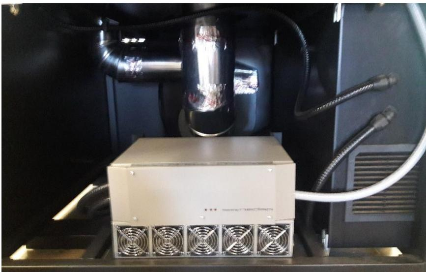
5. On the right side of the opening, towards the front of the conveyor, is a black-louvered fan cover. This cover can be removed by placing a flat-blade screw driver between the cover and the electrical housing and lifting the cover away from the housing (Figure 20).
