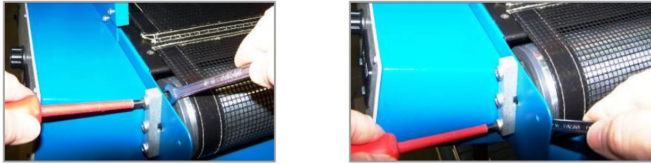
Figure 33. Loosening Drive-Roller Shaft-Support Fasteners
