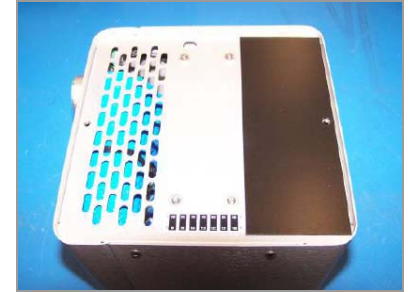
Figure 2. One Temperature Control Plate Installed
