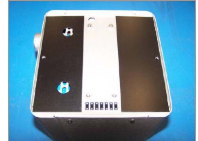
Figure 4. Two Temperature Control Plates Installed
