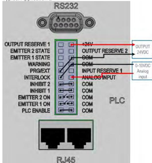
**Note:** The Input/Output terminal block is included in the packaging, with the jumper wires inserted. When the terminal block is installed, the controller will enter PLC mode. PLC mode disables commands and parameter settings from the HMI. To set parameters from the HMI, the terminal block must be removed, or the connection between the PLC Enable and COM pins (1 and 2) must be disconnected.
