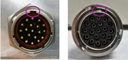
**Plugging the footswitch or light shield into the controller:**
