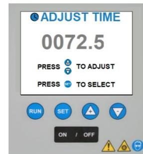
7. After the correct value is showing on the screen, press the **SET** Button.
