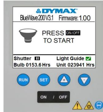
3. Turn on the internal UV Bulb by pressing the On Button located on the front panel.
