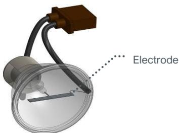
6. Install the new Bulb, plug the Bulb in and tighten the two Mounting Bracket Thumbscrews (Figure 43). Make sure that the center Electrode connecting the Bulb to the wire from the Reflector is parallel to the bottom of the system. Re-install the *BlueWave 200's* cover.
