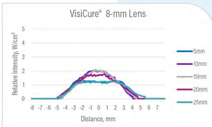
Note: Curing area data taken using Fuji UV Light Distribution Mapping System and normalized to ACCU-CAL™ 50 LED Radiometer.
