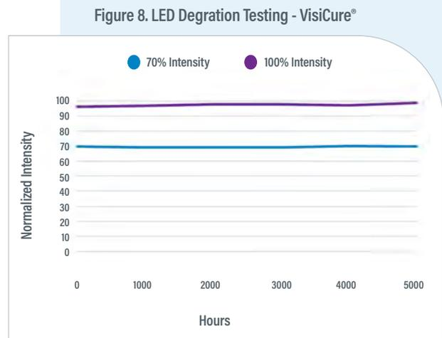
Note: Testing conducted at 70°F +/-3°F and 30% +/-10% Relative Humidity
